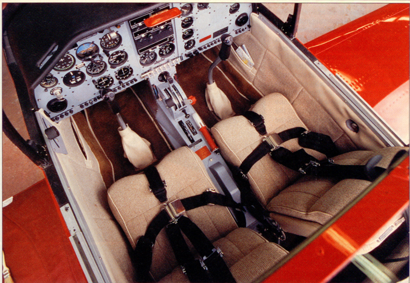
Pulling the large red handle atop the instrument panel (top) raises the rails of the jettisonable canopy (above, left).
