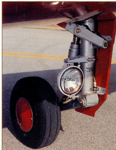
The trailing-link gear smooths ground handling and all but the worst landings.
