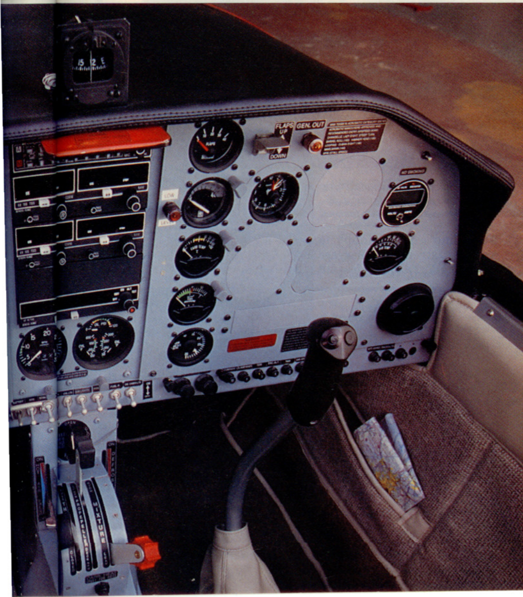
The F22B's tank contains 36 gallons of fuel behind the occupants' heads (above), which may cause a bit of concern in a crash. Dual throttles in both airplanes allow for left- or right-hand power management (below). A small baggage area resides behind the seats.
